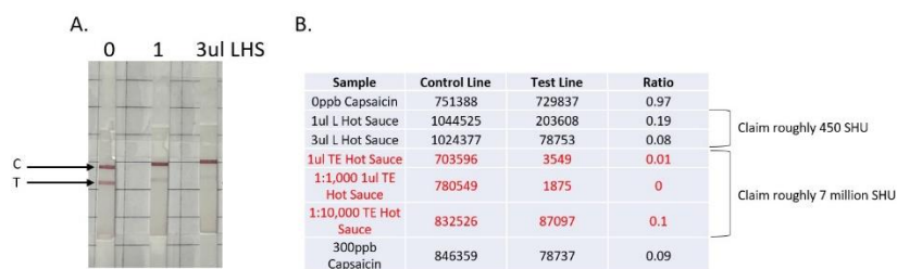
Figure 2. Evaluation of hot sauces using the Attogene Capsaicin Lateral Flow assay kit. Panel A shows the impact of a mild hot sauce on the test line of the lateral flow test. It can be easily visualized that both 1 and 3 ul of the LHS drastically reduced the test line indicating the presence of capsaicin in the sample. This intensity of the test line is like that observed with a capsaicin sample of 40ppb. We next tested an extremely hot – hot sauce (TE) and needed to significantly dilute the sample to start to observe a similar range as the LHS. Our estimation is that the TE hot sauce has at least 10,000x more capsaicin than the LHS. These data demonstrate the utility of using the capsaicin lateral flow test to detect and quantify capsaicin levels in hot sauces.
