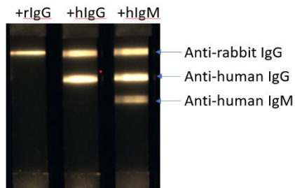
Figure 1. Biotinylated rabbit (r) IgG, human (h) IgG and human (h) IgM were sequentially mixed onto lateral flow running buffer. Next, strips that contained goat anti rabbit IgG (GAR), mouse anti human IgG or mouse anti human IgM capture lines were added into the well and run for 15 minutes. Results indicate a specific association of the capture lines with the desired biotinylated detector antibody using the universal lateral Human IgG/IgM lateral flow assay.
